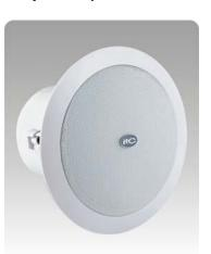
The T-208CW is a ceiling speaker built-in 70v/100v transformer. The 70v/100v transformer technique reduces line losses on longer distance and allows easy parallel connection of multiple loudspeakers.
